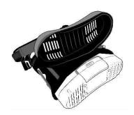
The Oxlife Liberty® is inserted into the carry bag from the bottom zippered section of the carry bag.
