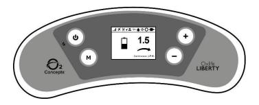
When the device is powered on it will enter a five (5) minute warm-up period to reach desired performance. The warm-up period is indicated on the display screen by a green ring that becomes a green circle once warm up is complete.
